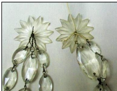
CRYSTAL RESTORATION provided new challenges. Re-wiring of the swags provided additional challenges, due to their varying weights, each crystal required a unique wiring procedure. After cleaning and repair, each crystal chain had to be “rinsed.” Broken crystals were repaired or replaced.
